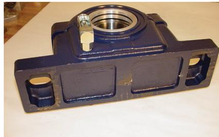
Rugged Base Provides for Superior Housing Strength and Allows for Oil Equalization Slots Under Bearing Seat. This Ensures a Balanced Oil Level on Each Side of the Bearing.
