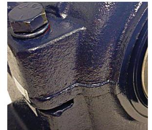
Pry Slots Allow for Easy Cap Removal.
